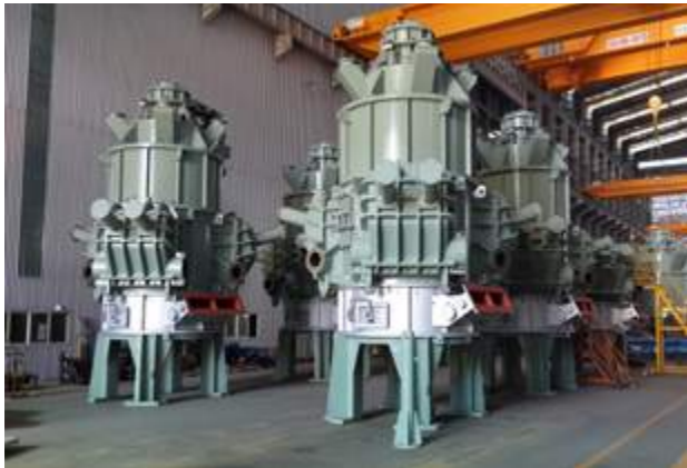
Pulverizer(600MW Coal Fire Power Plant)
