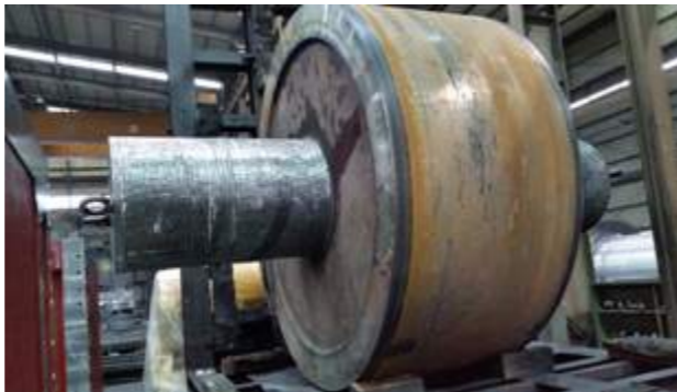
Crusher Roll(65tons, Forged Steel+hard facing)
