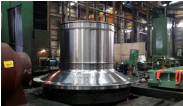
Trunnion Mill Head(47tons, Cast Steel)
