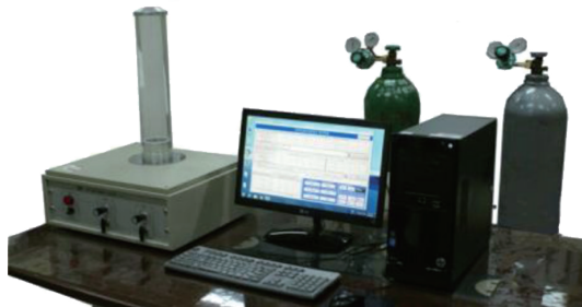
Oxygen Index Tester ISO 4589-2
