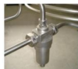
safety function in the pressure regulator
