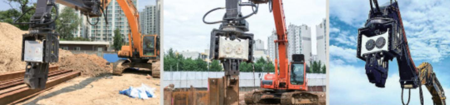
Vibratory Hammer (Pile Driver) is an useful machine of excavator.
