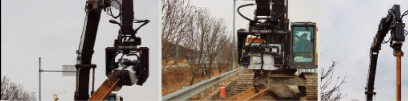
Vibratory Hammer (Pile Driver) is an useful machine of excavator.
