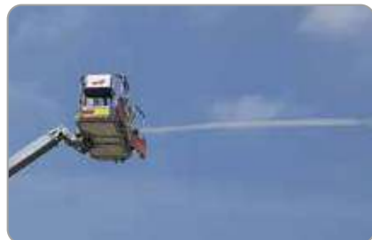
Automatic water turret operations (Spray / Jet)
