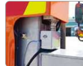
Outrigger Jack detection sensor and Safety Check-Valve
