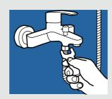
Remove the screw of the shower hose connected to the shower faucet by a spanner.
