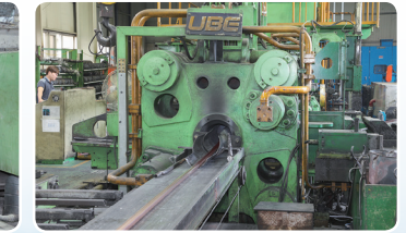
2,750-ton Extruding Machine
